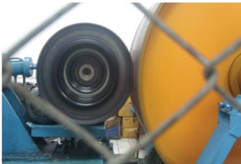
Tyron ATR undergoing load and speed testing
