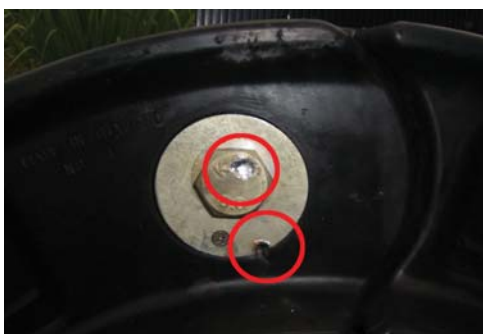
Minimum impact damage to runflat fixings
